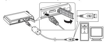
The camera is automatically turned on and the poweron lamp will light or blink. The camera monitor will remain off
